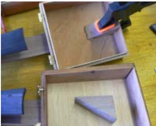
Installing the tail block.
