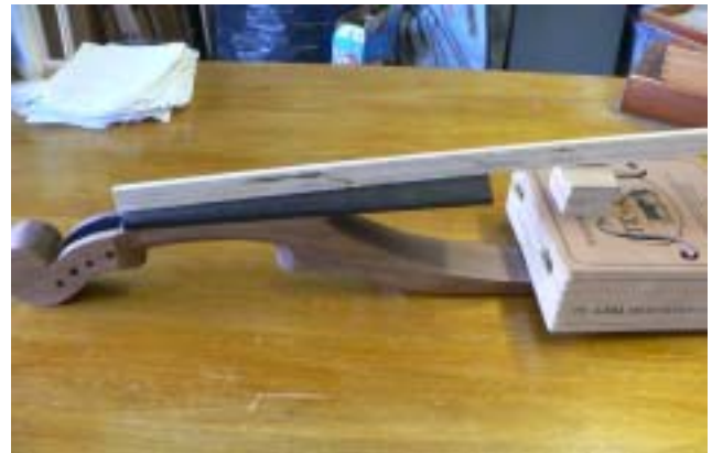
Checking the string path and bridge position.
