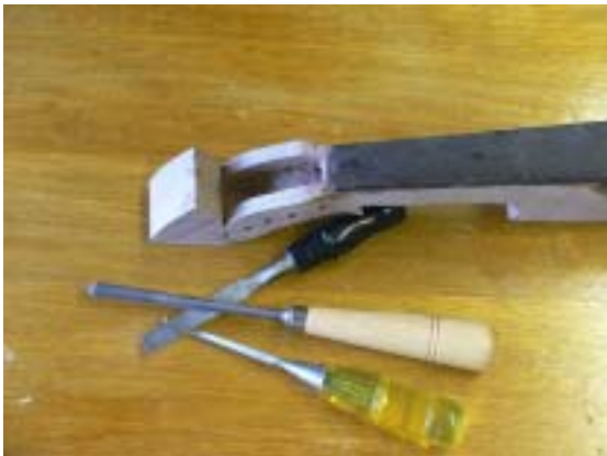
Hollowing out the peg box.
