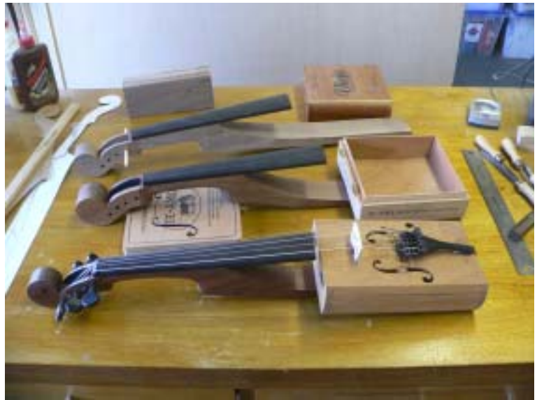
Bridge, strings and tailpiece are installed.
